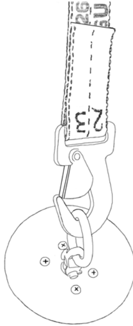
Figure 2-29 – Belt Assembly Clipped to Cargo Ring
