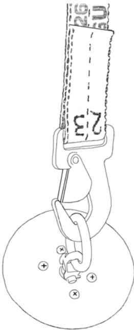
Figure 3-13 – Belt Assembly Clipped to Cargo Ring
